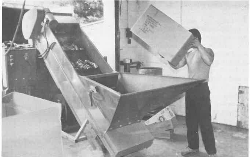
The Rockaway Valley Paper Recycling Center, in Wharton, buys aluminum cans. Here, an automatic can-collator removes contaminants, flattens cans, and blows them into a trailer.
