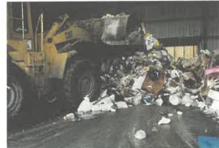
At the Mt. Olive Transfer Station, a front-end loader pushes waste towards the tunnel where a tractor-trailer is parked. When the tractor-trailer is full, the waste will begin its journey to Pennsylvania for disposal.
