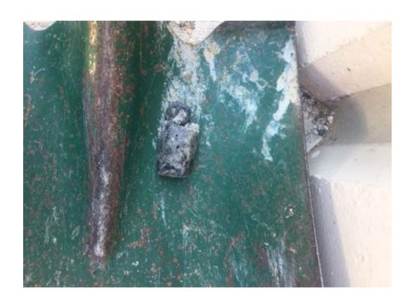
This lithium-ion battery was removed from the tip floor by a wheel loader and extinguished immediately.
