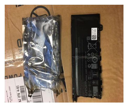
This laptop battery was spotted on the incline belt by a loader. It was successfully extinguished by presort personnel.
