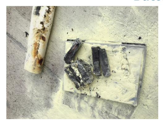
This battery was found after the baler ejected the bale. It was sprayed immediately and continuously until the smoke subsided.
